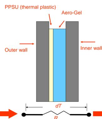
The thermal resistance is defined as the ratio of the temperature difference,  $dT$ , to the heat transfer  $Q$ . Ohm's law states that the electrical resistance is defined as the ratio of the voltage drop across a resistor to the current flow across the resistor. The insulation from the PPSU and the aero-gel acts as a resistor.
