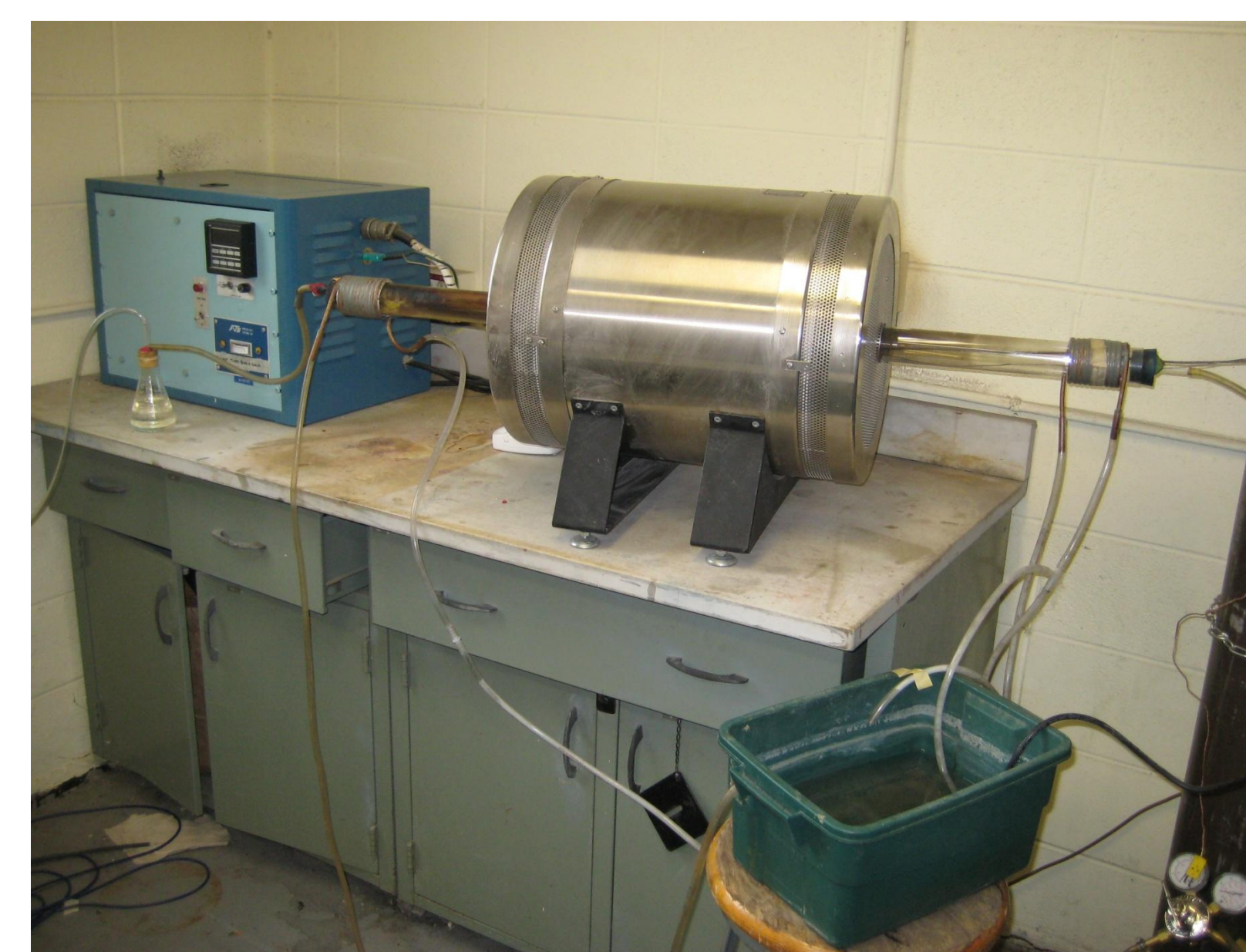
Figure 2 . Image of quartz tube furnace setup.
