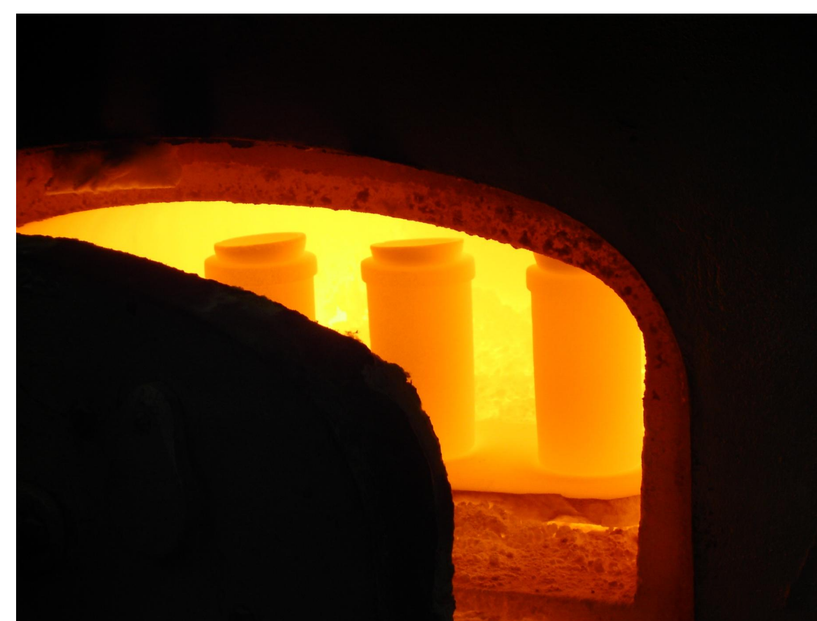
Figure 1 . Image of crucibles in muffle furnace during first reduction test.
