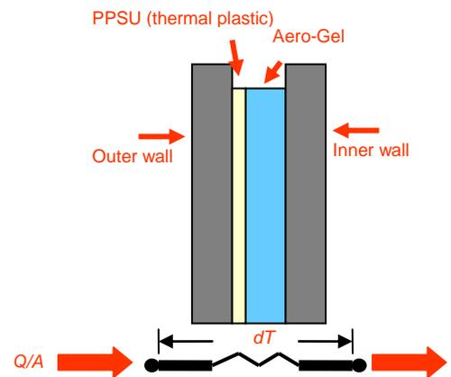
Figure 1 - Thermal Resistance Model
