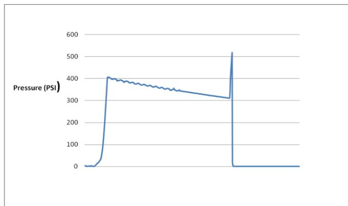
Figure 5 – Pressure Curve Hydrostatic Burst Test
