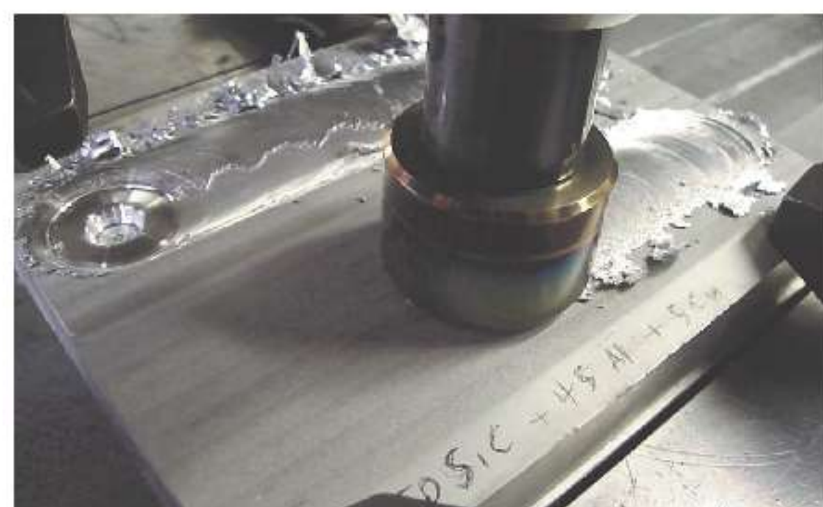
Figure 9. The FSW process
