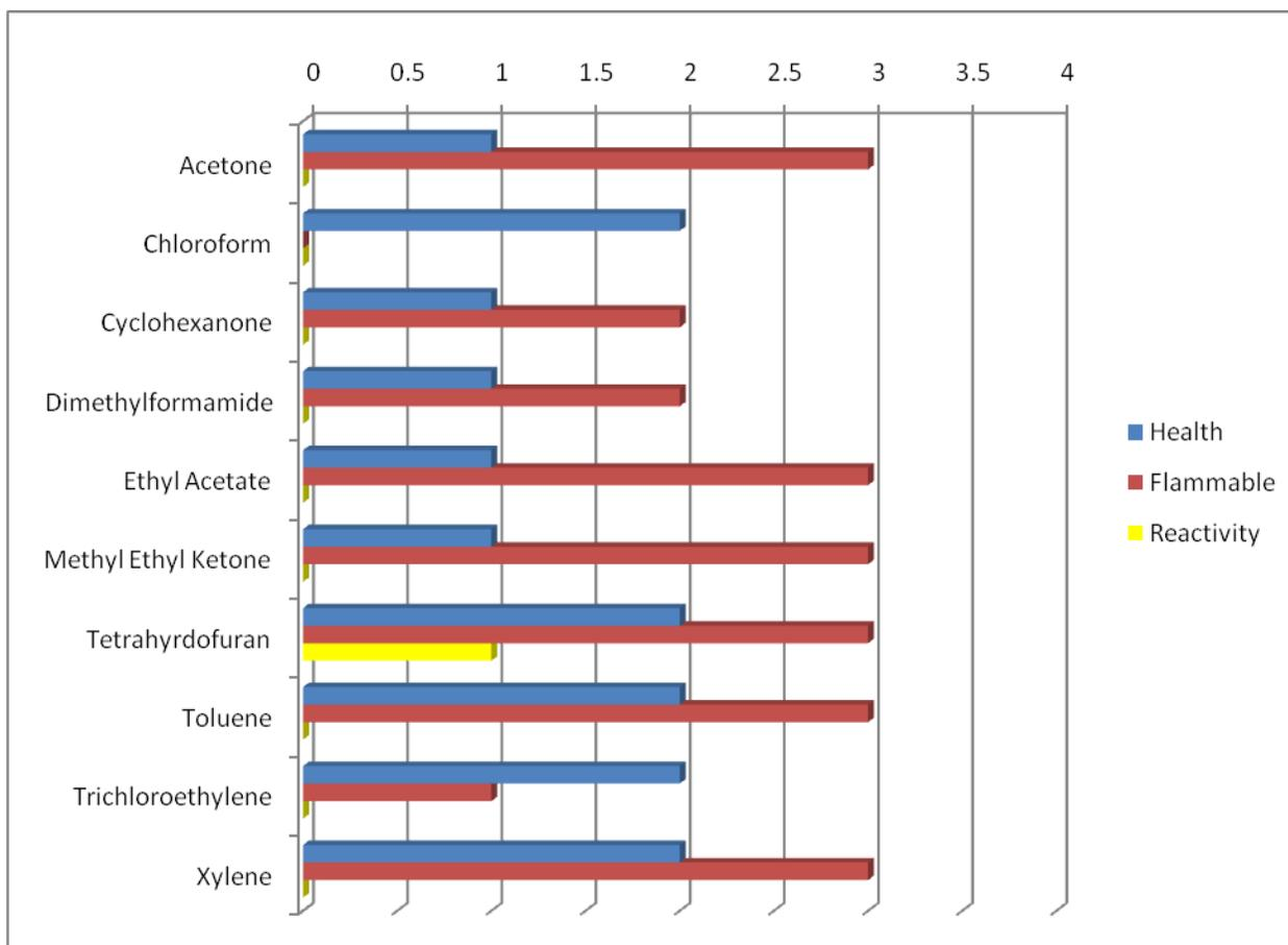
Figure 3: NFPA 704 Chemical Hazard data for considered and experimentally used solvents. [8-17]
