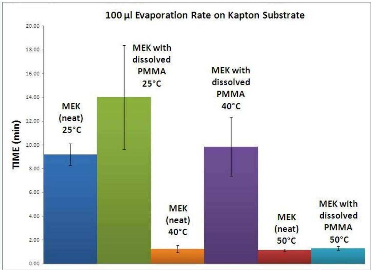
Figure 6: Evaporation rates of drop-tests of MEK (neat) and MEK with dissolved PMMA. [20]
