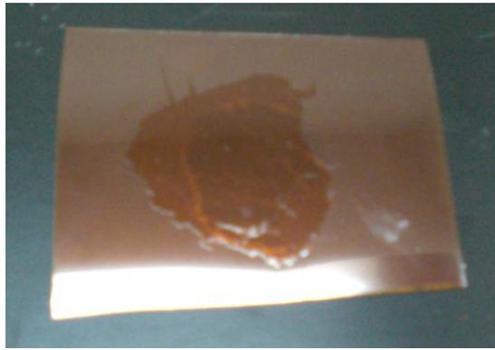
Figure 5: Kapton substrate showing fully evaporated drop-test. [19]
