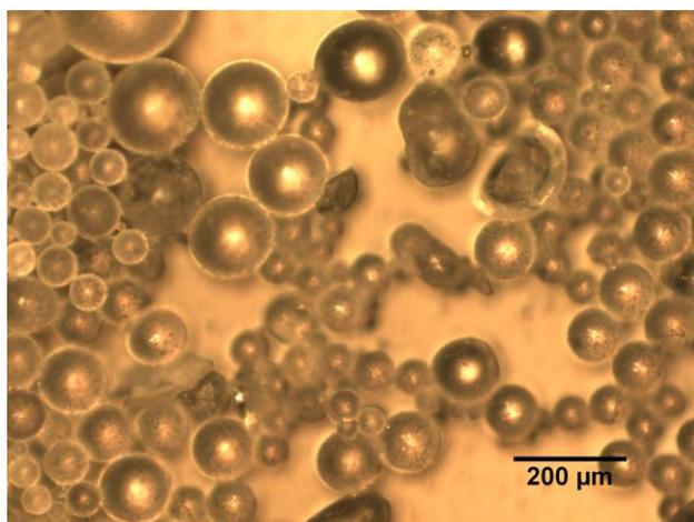
Figure 1: Powder PMMA at 10x reveals spherical particles, below 300μm in diameter. [2]
