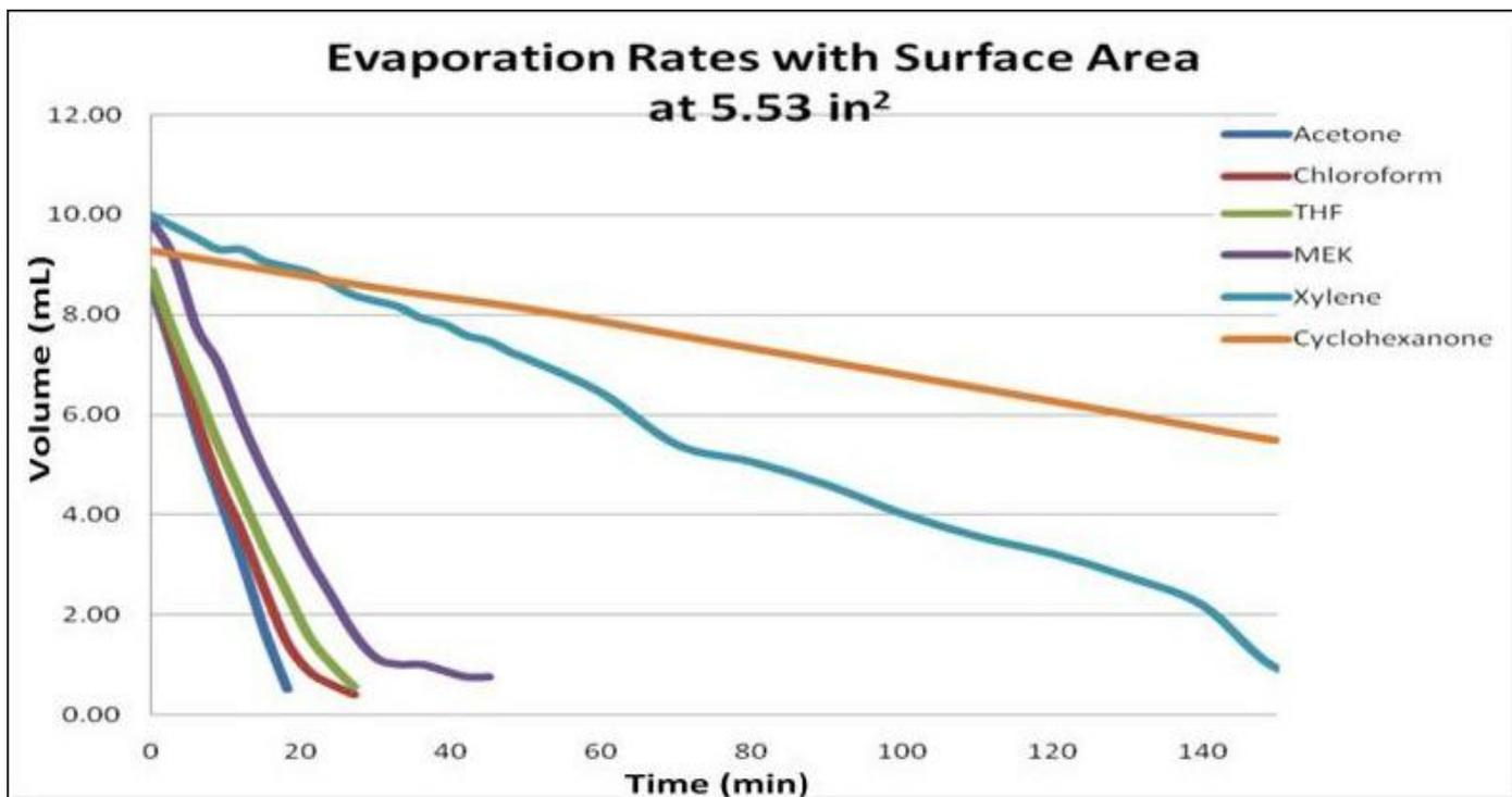
Figure 2: Plot showing evaporation rates for all solvents involved in trial 2. [6]
