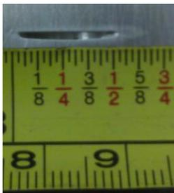
Figure 4: Fatigue Crack Width
