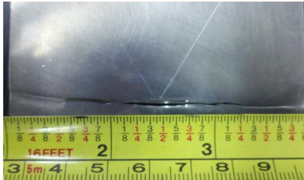
Figure 6: Failure of an Un-Repaired Sample
