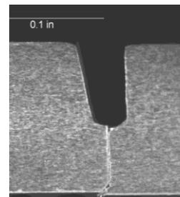
Figure 5: Fatigue Crack Macro (side)
