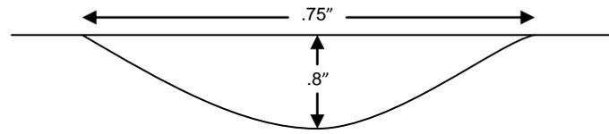
Figure 3: Pre-Crack Dimension (front)
