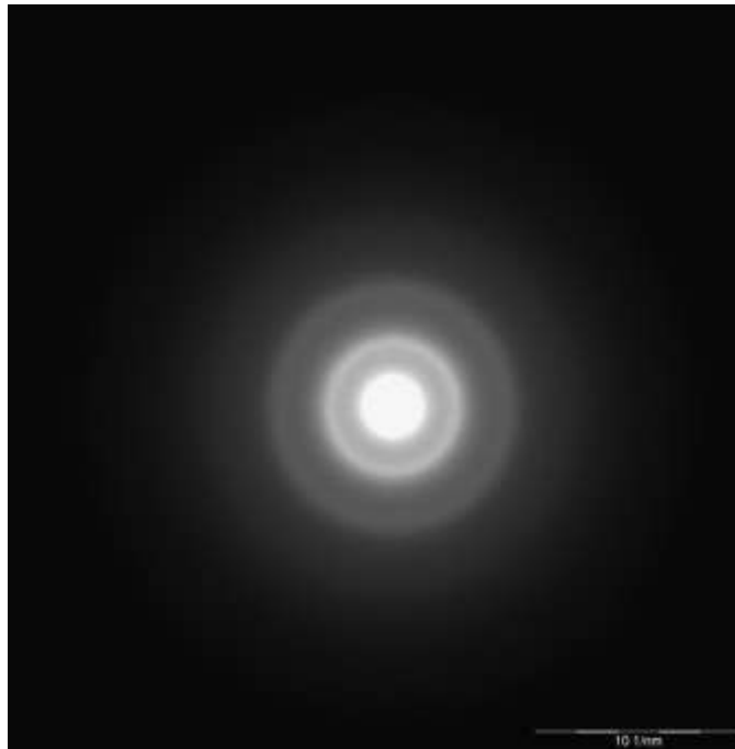
Figure 4: Sample A2, amorphous diffraction pattern prior to heating
