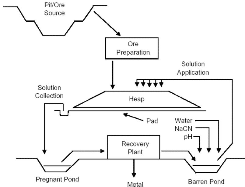
**Figure 16: Heap leaching schematic according to e-gold prospecting.**
