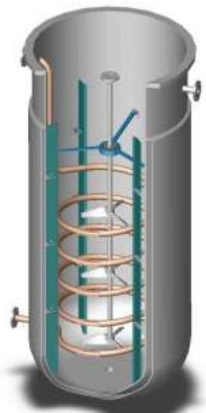
**Figure 17: Vat leaching schematic.**
