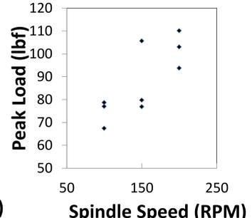
Figure 16: Peak load vs. spindle speed with a constant plunge rate of 2 in/min for PC.
