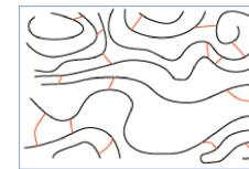
Figure 6: Schematic of a crosslinked polymer network
