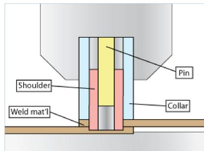
Figure 2: Schematic of the side view of the refill FSSW process
