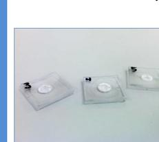
Figure 14: FSSW on polycarbonate.
