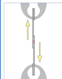
Figure 10: Schematic of a lap shear test
