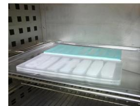
Figure 9: Silicone molds in oven
