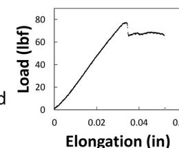
Figure 11: A representative PC load vs. elongation graph from lap shear testing.
