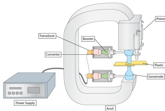
Figure 1: Schematic of Sonobond ultrasonic spot welder at SDSMT
