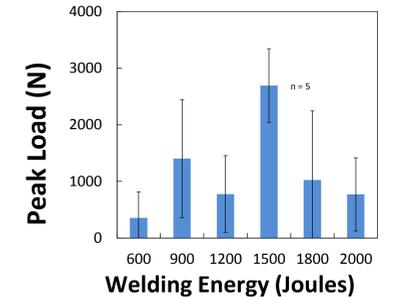
Figure 12: Peak loads of USSW of 1/8" PC from lap shear testing. Error bars represent one standard deviation. (Navaraj Gurung)
