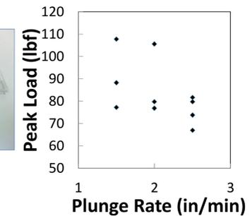
Figure 15: Peak load vs. plunge rate with a constant spindle speed of 150 RPM for PC.
