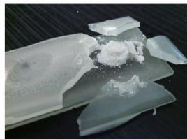
Figure 13: FSSW of epoxy.
