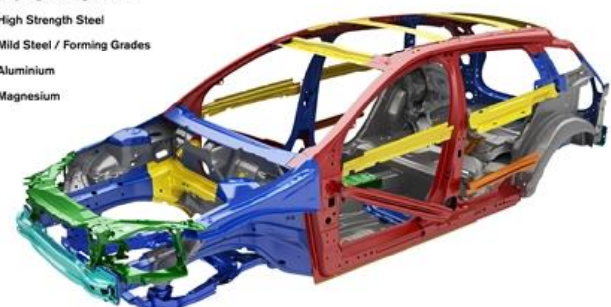
Figure 3: Example of Aluminum and Magnesium Alloys used in cars to reduce weight http://boronextrication.com/files/2012/05/2010_Volvo_V60_Body_Structure_Safety_Cage_Extraction_UHSS_Boron.jpg
