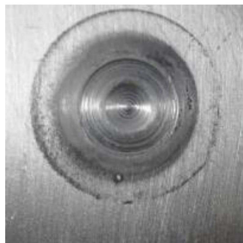
Figure 1: Friction Stir Spot weld using sleeve plunge sequence
