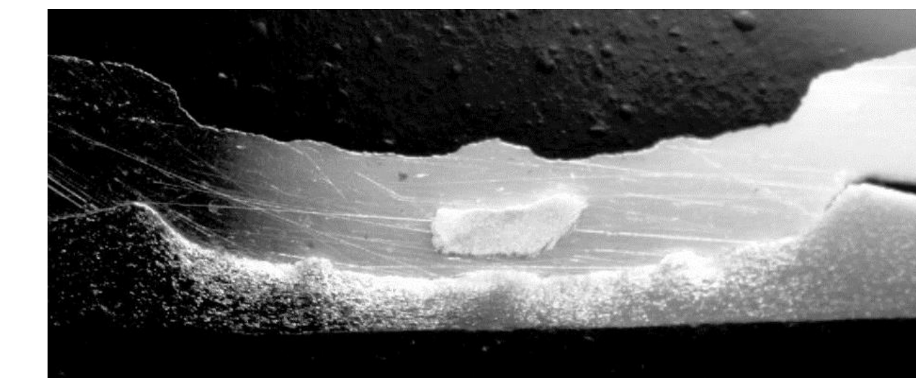
Figure 8 : Macro of the cross section of a weld made using the sleeve plunge weld sequence
