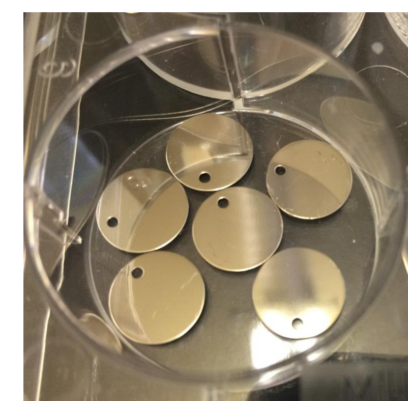
Figure 2: Blank Ti samples prepared for anodization.
