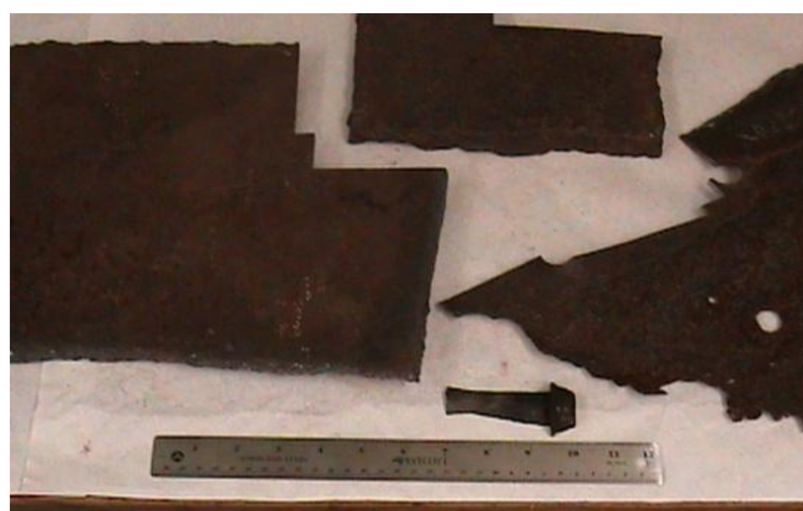
Figure 1: Photograph of the selected steel pieces from the U.S.S. Arizona at Waipio Point. Left: Plate A-1. Top: Plate A-2. Right: Plate A-3. Bottom: Rivet.
