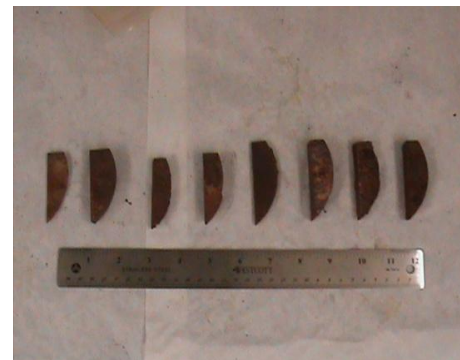
Figure 6: Photograph showing the core samples taken from the U.S.S. Arizona.
