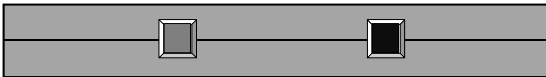
Figure 2. – Aluminum tubes packed with aluminum powder and carbon nanotubes between two aluminum plates.
