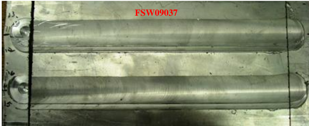
Figure 6. – Welds 11-13 are Al powder and welds 14-16 are SWNT.
