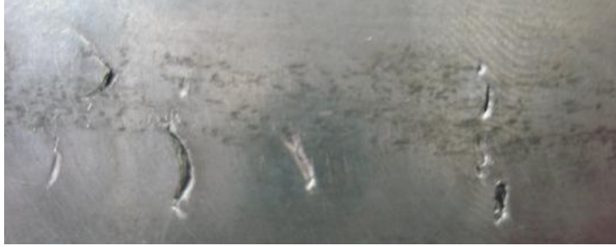
Figure 8. Cracks formed on bottom of the rolled SWNT sample after a 50% reduction.
