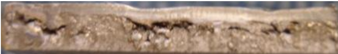
Figure 14. – Voids on the edge of the nugget post shearing.
