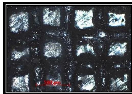
Figure 2. Ti-15Mo Grid used for cell culture
