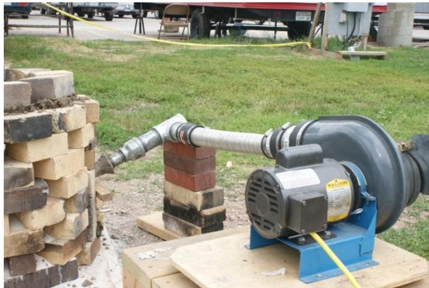
*Figure 3- Furnace air supply equipment*
