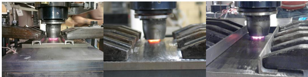
Fig. 11: Cast iron welds with different clamping methods
