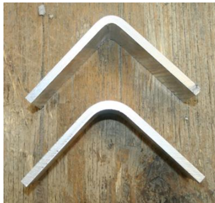
Figure 9 Top Figure represents a FSP angle and bottom is a Traditional formed angle.
