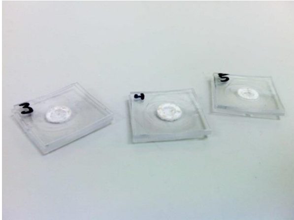
Figure 12: An Example of FSSW on 1"x 1" PC (Author's Work)
