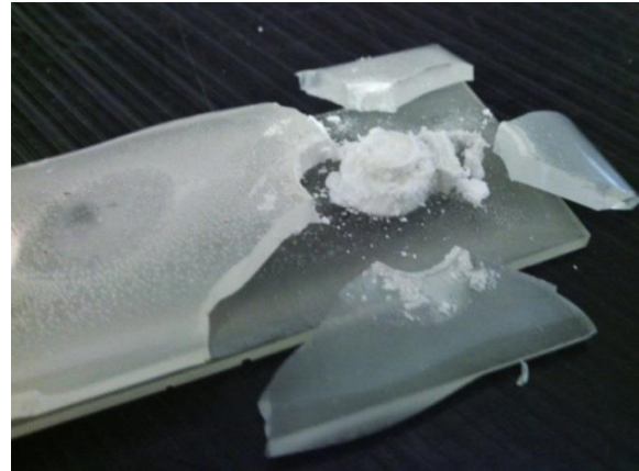
Figure 13: FSSW on Epoxy. The short dimension of the original epoxy sample is 1" wide. (Author's Work)
