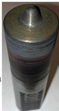
Figure 2: Tungsten rhenium hafnium carbide tool
