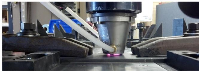
Figure 1: Friction stir welding of high strength steel
