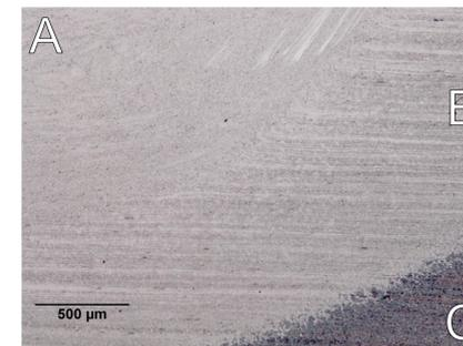
Figure 6: Layers of weld material at 7ipm.
