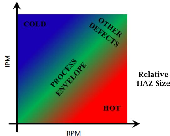
Figure 3: Graphical representation of balancing weld parameters
