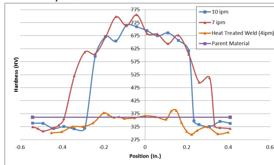
Figure 5: Microhardness traverses of different weld parameters
