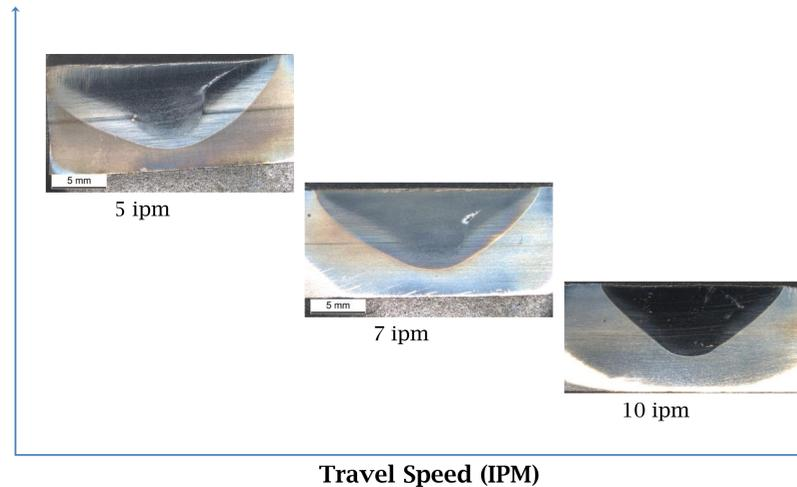
Figure 4: Decreasing HAZ size with lower heat input
