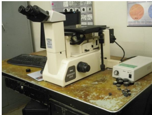
Figure 7: Optical Microscope with mounted sample
