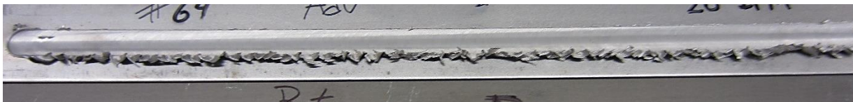
Figure 15: Weld showing excess amount of flash.
