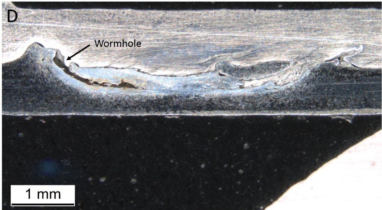
Figure 9: Macrographs of welds 64-67 made with tool A and coated steel. A) weld 64 Aluminum advancing 20 IPM B) weld 65 Aluminum advancing 30 IPM C) weld 66 Aluminum retreating 20 IPM D) weld 67 Aluminum retreating 30 IPM.
