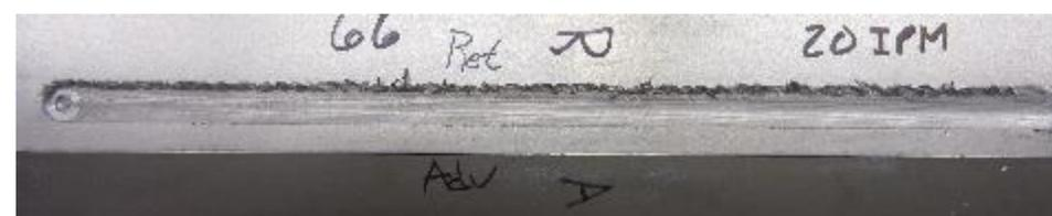
Figure 3. Weld made with scribe tool.
