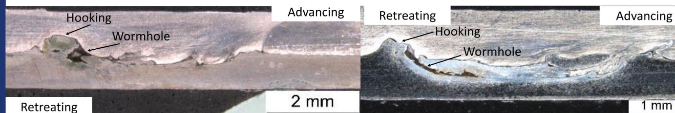
Figure 2. Welds 66 and 67 macrographs respectively
