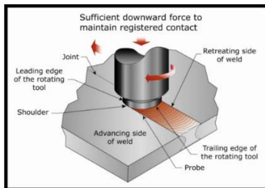
Figure 1. Diagram of FSW process (www.twi.co.uk)
