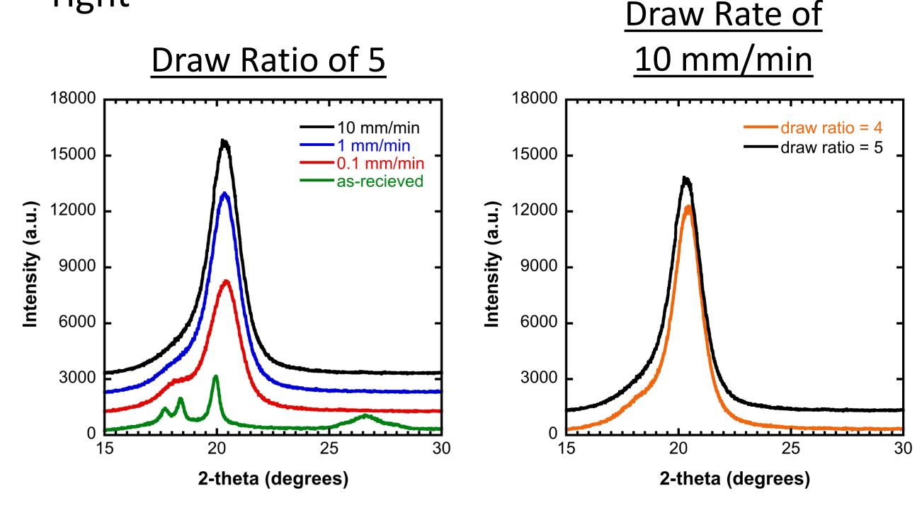
The β-phase was most defined when drawn at a temperature of 80°C with a draw rate of 10 mm/min and a draw ratio of 5
