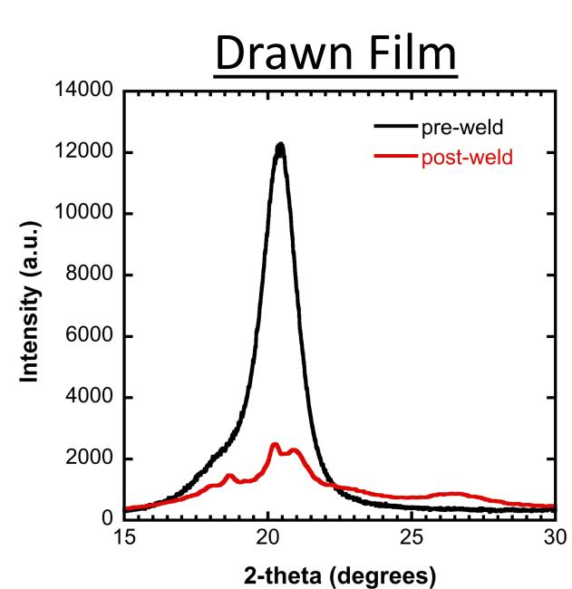
The welded drawn film shows increasing peaks at 17, 18, and 26 degrees, indicating that the welding has transformed the PVDF back into the  $\alpha$ -phase
