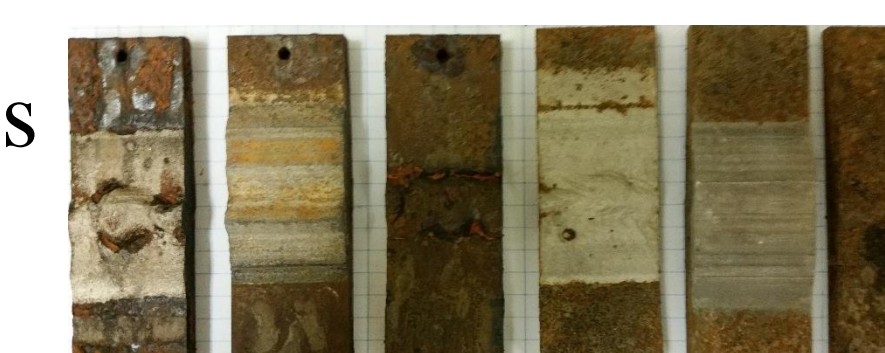
Figure 9: Removal after 10 day exposure (after cleaning)
