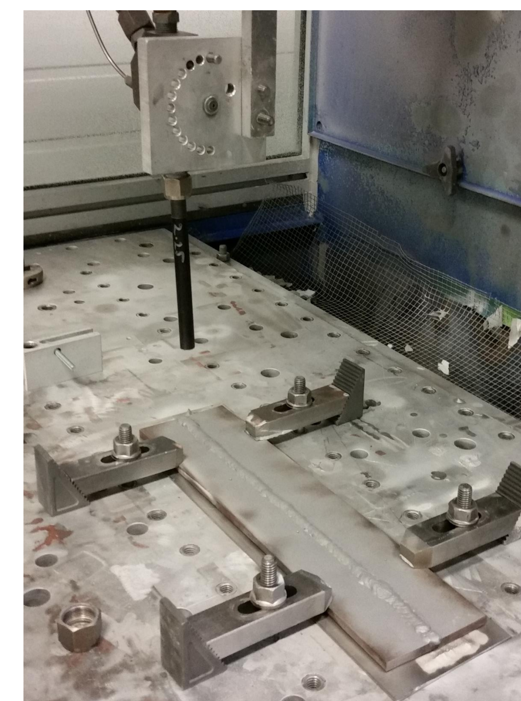
Figure 3: Steel plate being cold sprayed with 6061 Aluminum
