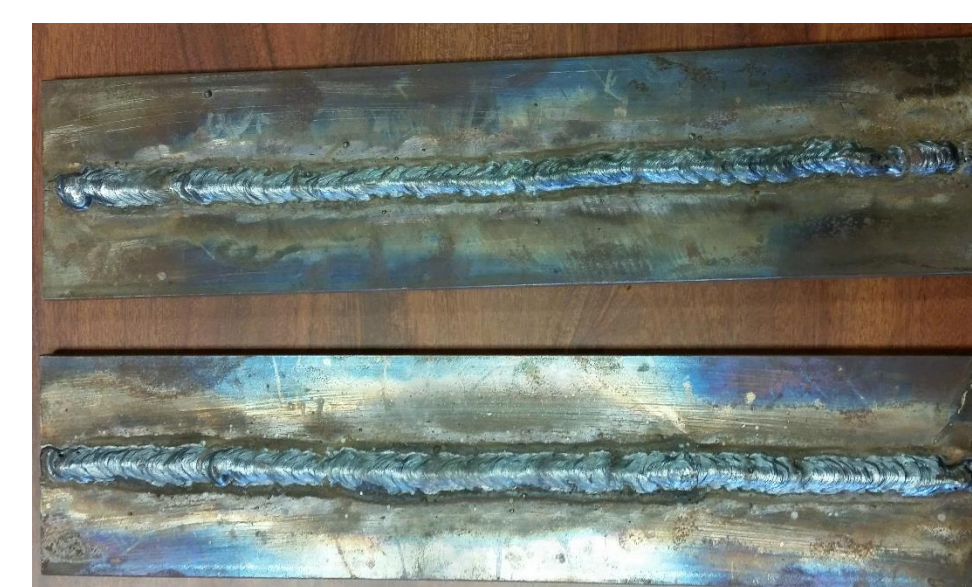
Figure 4: Steel plates after welding (before spray)
