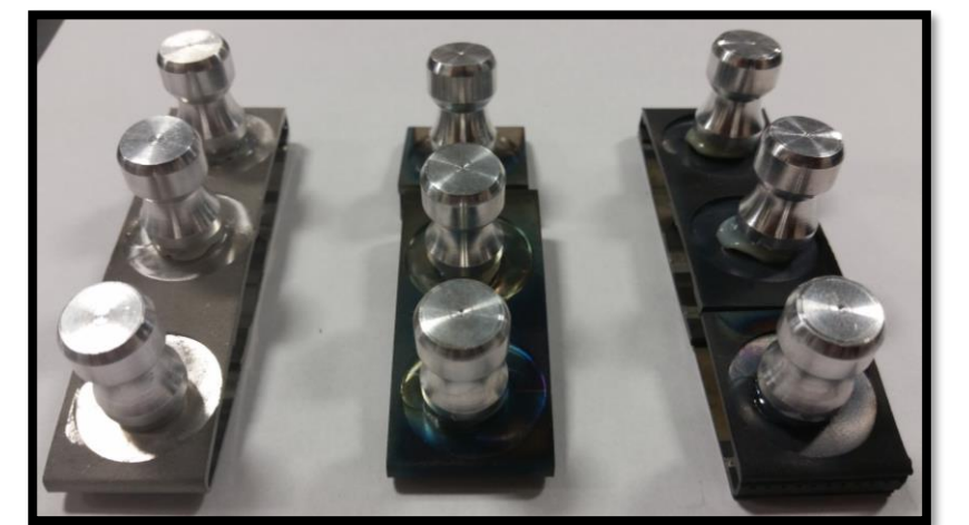
Three samples with mating caps attached. Each post spray condition is tested for bond strength three times.
