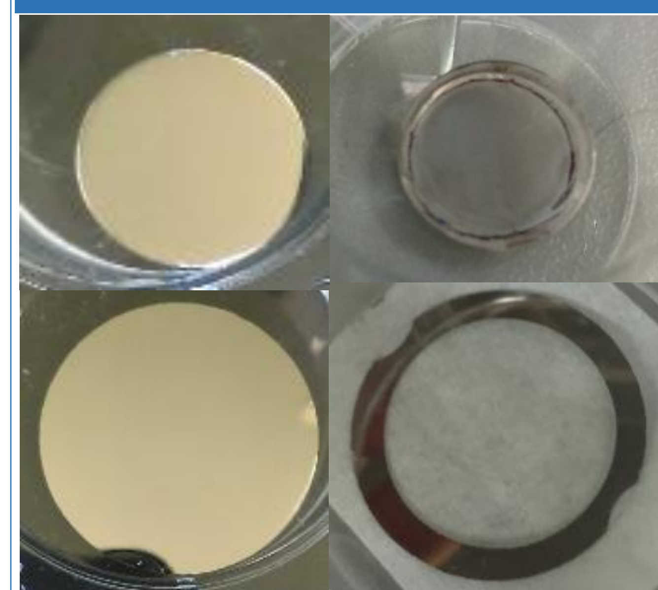
Top: Opaque samples before and after anodization Bottom: Transparent samples before and after anodization
