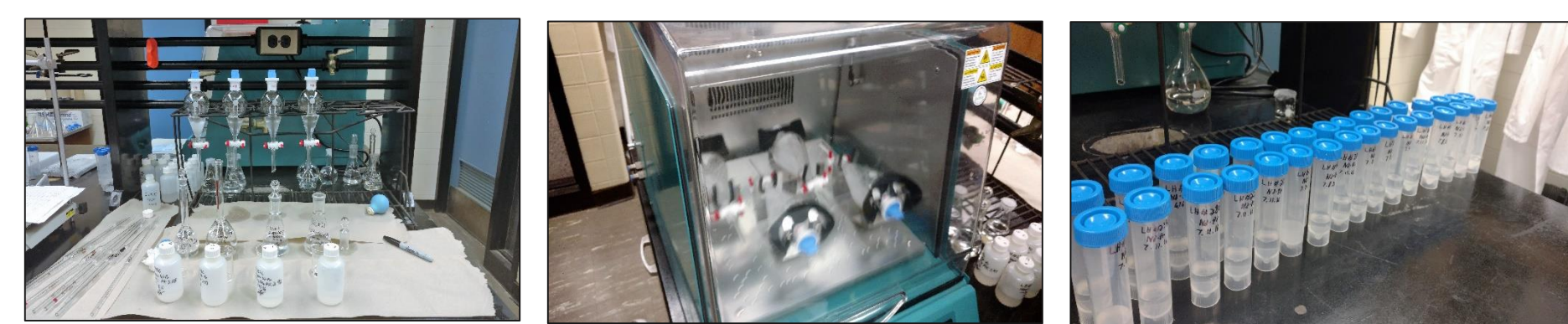
Figure 1. The Process in Pictures: (left) Setting up a solvent extraction set, (middle) Shaking Separatory Funnels, (right) Final experiments
